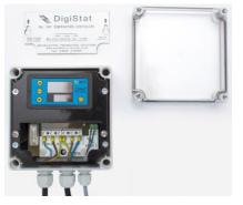
Install the flexible cable leading to the controlled load via the centre cable gland and connect to the right hand grey terminal block marked "LOAD OUT". Live (Brown) to L, Neutral (Blue) to N, Earth (Green/Yellow) to E.
